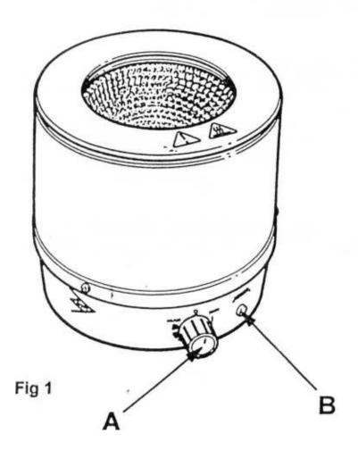
A = Mains on/off & power control knobB = Load indicator
