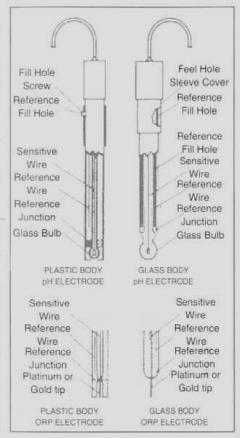
For a faster response lower the rubber sleeve (or unscrew the fill hole screw).
