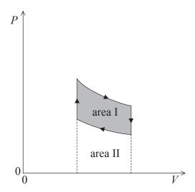
Which of the following area(s) is/are equal to the work done by the gas as it expands?
