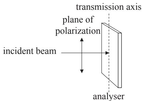
The angle between the transmission axis of the analyser and the plane of polarization of the light is  $\theta$ . In the position shown the transmission axis of the analyser is parallel to the plane of polarization of the light ( $\theta=0$ ).
