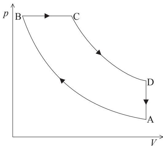
AB and CD are adiabatic changes of state. The pressure at point B is  $1.8 \times 10^5 \text{ Pa}$  and the change in volume of the gas between B and C is  $4.8 \times 10^{-4} \text{ m}^3$ .
