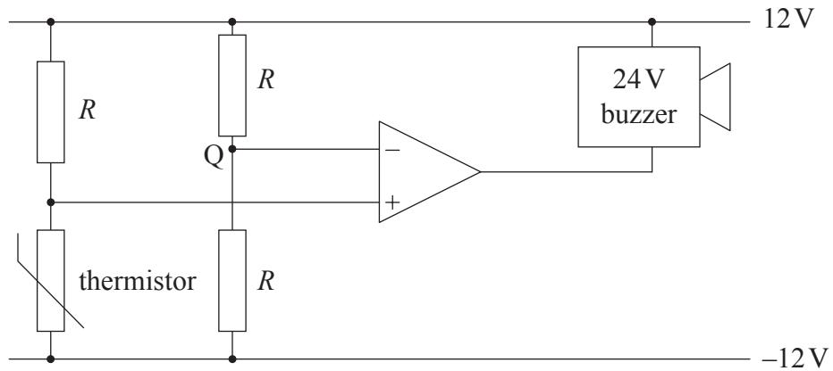
It is required that the buzzer should sound when the temperature of the thermistor rises above 50°C.
