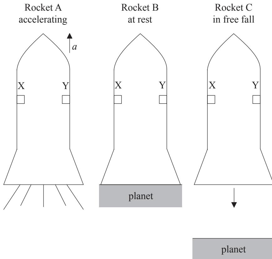
Rocket A is accelerating in outer space with acceleration  $a$ .
