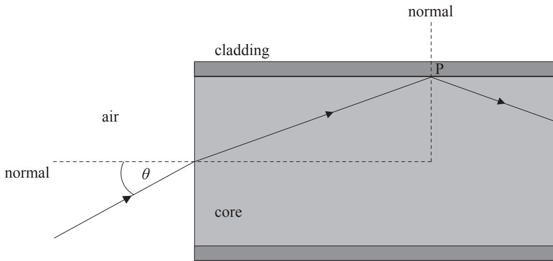
The refractive index of the core is 1.56 and that of the cladding is 1.38.
