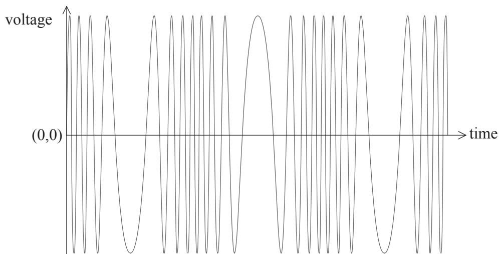
The carrier wave is modulated by a single frequency signal.
