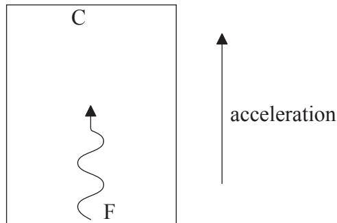
A monochromatic beam of light is emitted from the floor F of the rocket. The beam is received at the ceiling C of the rocket. Suggest why the frequency of the light beam measured at C is less than the frequency measured at F.
