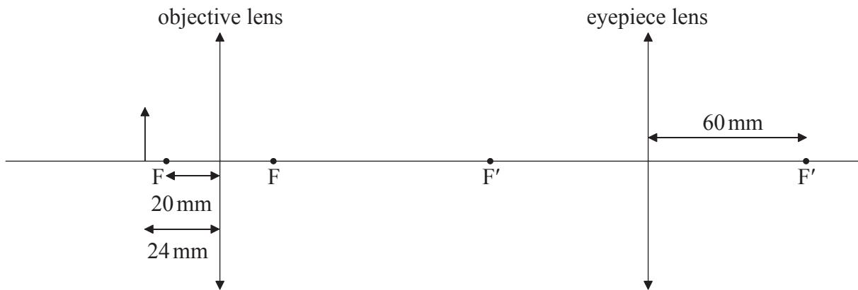
The focal length of the objective lens is 20 mm and that of the eyepiece lens is 60 mm. A small object is placed at a distance of 24 mm from the objective lens. The microscope produces a final virtual image of the object at a distance of 240 mm from the eyepiece lens.
